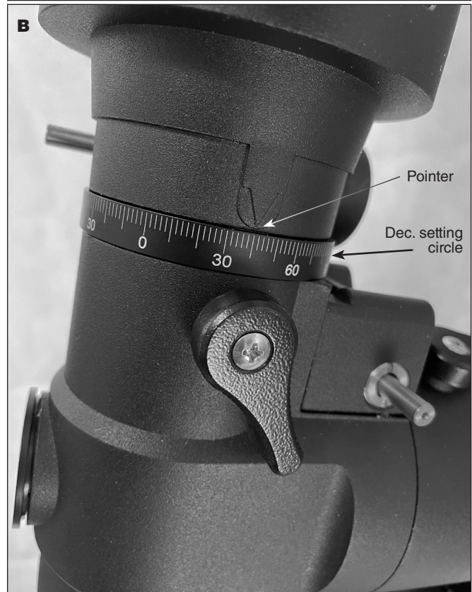
Figure 16 A.) The polar scope and R.A. setting circle. B) The Declination setting circle.
