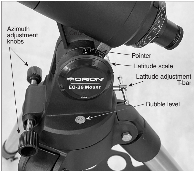
Figure 14. Features for leveling the mount and adjusting its latitude and azimuth positions.
