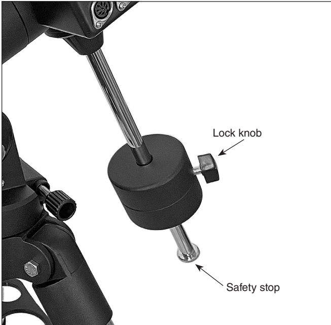
Figure 7. Install the counterweight, then make sure the “toe saver” safety stop is threaded on.
