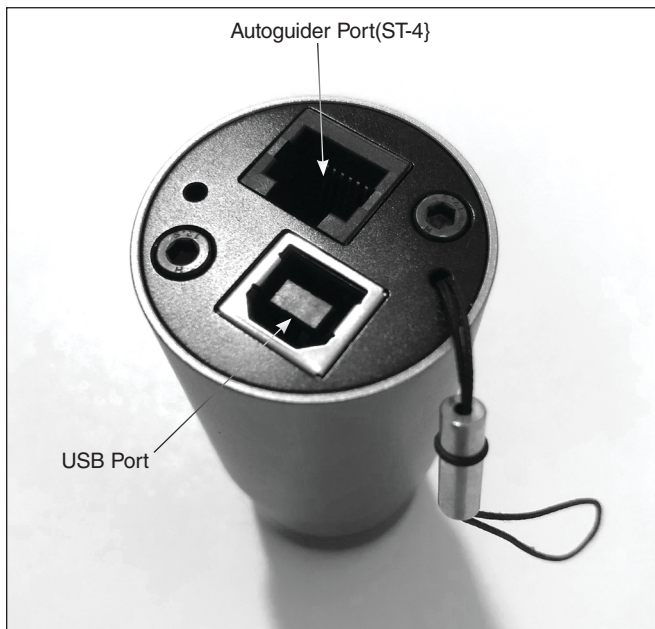
Figure 5. The USB and autoguide ports of the StarShoot Mini Autoguider.
