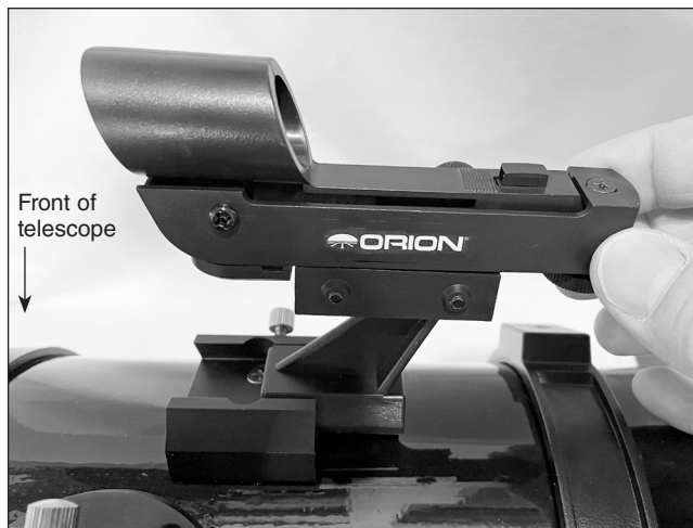
Figure 8. Slide the EZ Finder II into the telescope's finder scope base as shown.
