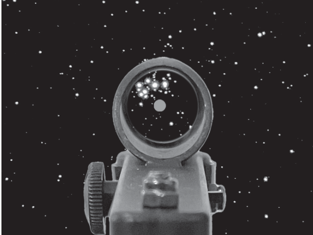
Figure 23. The red dot scope superimposes a red LED dot onto the night sky, showing right where your telescope is pointed.
